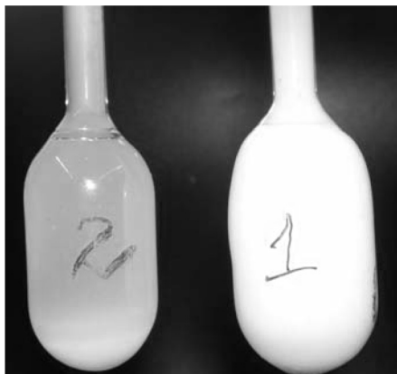
FIGURE 1 The photography of dilatometers with reaction mixtures obtained in the processes of block copolymerization of PAAc with MEPEG3-1 and AAc homopolymerization-2.
